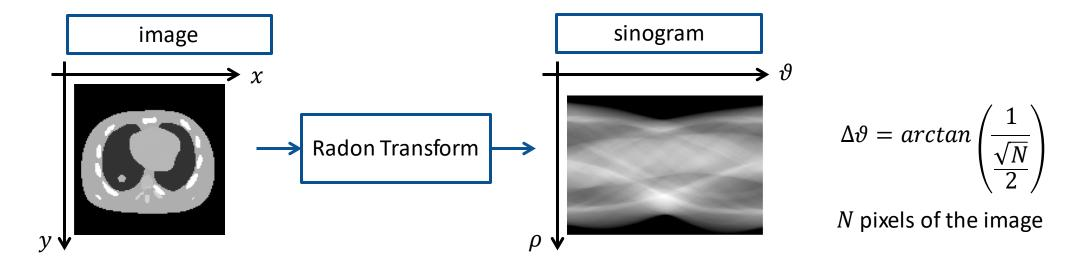
The Fourier Slice Theorem, provided with the Nyquist theorem of sampling, enables the implementation and application of analytical reconstruction algorithms (i.e., the filtered back-projection)
