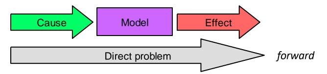
• The solution of the inverse problem requires the mathematical model of the direct problem that links cause-effect of a certain phenomenon to explore the parameter space of the causes (i.e., solve the problem by finding the causes of the phenomenon, when the causes are not directly observable)
