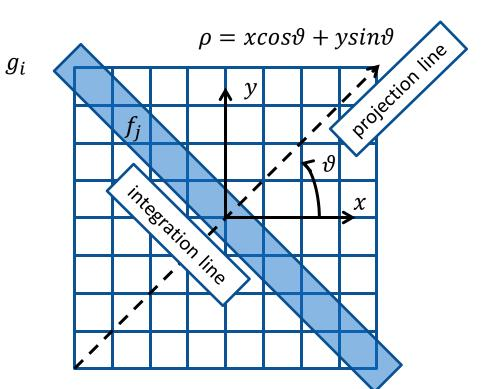
The coefficients a<sub>ij</sub> (i.e., the elements of the system matrix) express the intersection area/volume of the pixel/voxel j with the integration line of the projection i
