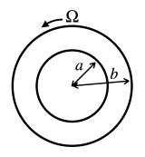
Consider a slow, steady laminar flow in an annulus between an inner cylinder of radius a, which is at rest, and a concentric outer cylinder of radius b, which is rotating about its axis with angular velocity  $\Omega$  (see figure above).
