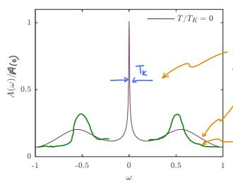
NRG correctly captures width of central peak around  $\omega = 0$ , the 'Kondo resonance'.
