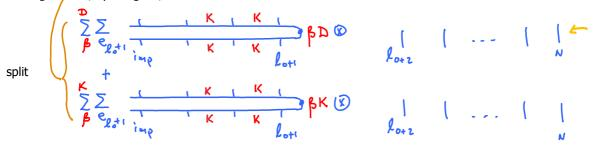
Iterate until the entire chain is diagonal, and declare all states of last iteration as 'discarded':
